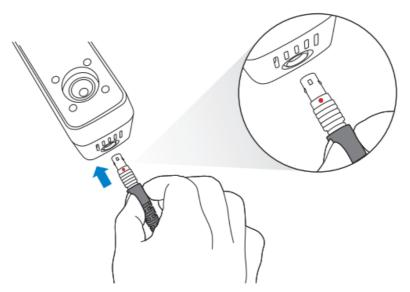
2. Plug the power cable into the USB cable.
